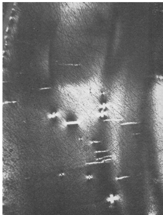
Figure 1 The strain associated with iridium inclusions and filament defects as viewed in polarized light ( \times 45 ).
