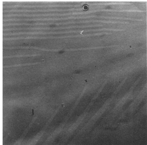
Figure 6 The effect of the substrate core on a film of (Y\text{Gd})_3(\text{GaFe})_5\text{O}_{12} which is only just capable of supporting bubbles ( \times 220 ).
